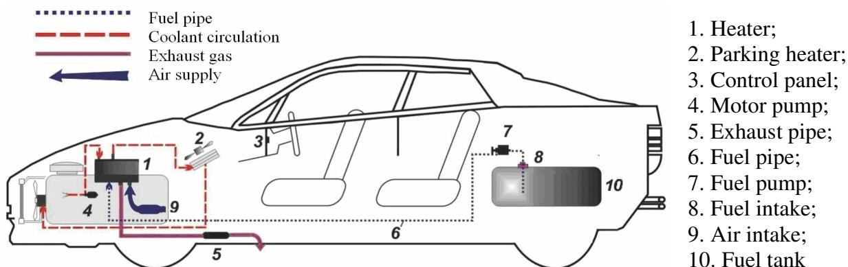
Figure 7.1 - Pre-heater installation diagram
