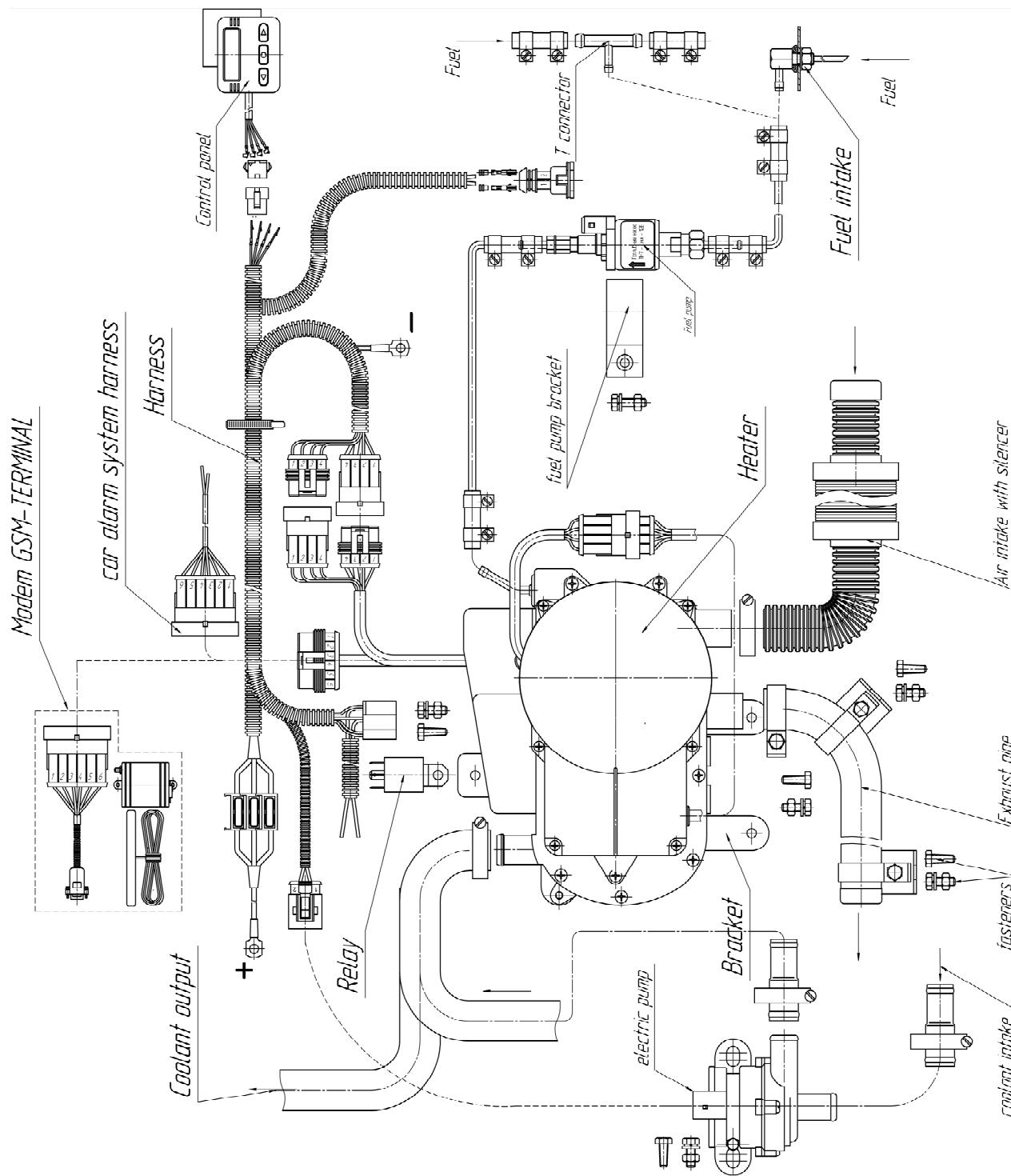
Figure 4.2 – Pre-heater basic components
