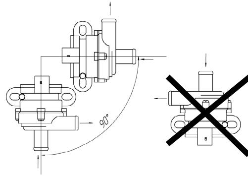
Figure 7.4 – Recommended position of the motor pump
